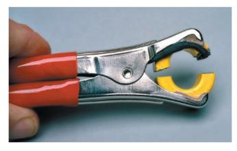
This view of the completed current clamp clearly shows the general arrangement. If the toroid core becomes magnetised during use, it can be demagnetised by momentarily reversing the current flow in the core.
