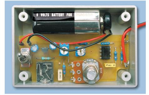
There's plenty of room inside the case for the PC board and a 9V battery. The board is held in position by slipping the case lid over the switch and pot shafts and doing up the nuts.
