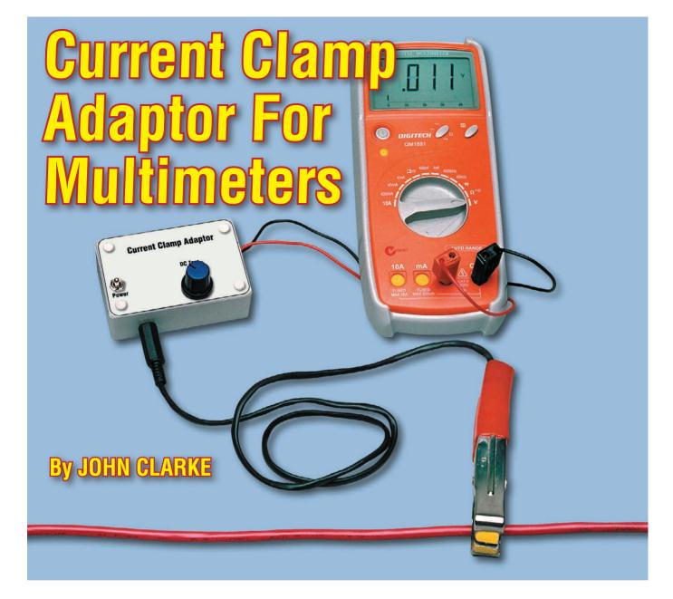
Looking for a current clamp meter that won't break the bank? Here's a simple clamp meter adaptor that you can build for about £15. It plugs into a standard DMM and can measure both AC and DC currents.
