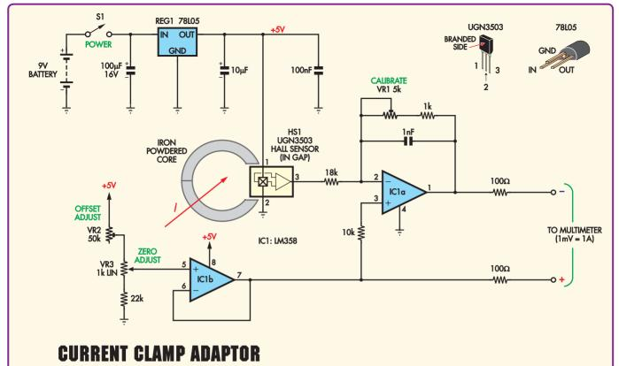
Fig.1: the circuit uses Hall effect sensor HS1 which produces a voltage at its pin 3 output that depends on the magnetic field induced into an iron-powdered toroid core. This voltage is fed to op amp IC1a which then drives the negative terminal of the multimeter. IC1b drives the meter's positive terminal and provides null adjustment.
