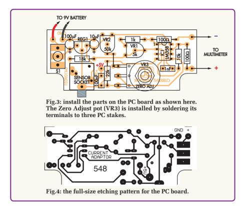
set to mid-range, so that the multimeter reads 0V with no magnetic field applied to the Hall sensor. VR3 is then adjusted during subsequent use of the clamp meter—it can vary IC1b's output by about 25mV to null out any small voltage readings.
