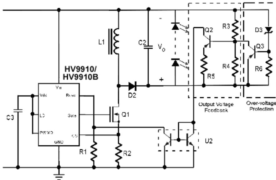
In a Buck-boost converter without the output voltage feedback, the output current is proportional to the ratio of the switching frequency to the output voltage. The feedback circuit makes the switching frequency proportional to the output voltage making the LED current constant over varying LED string voltages.
