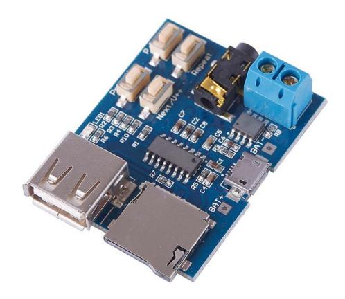
This MP3 decoder board can play MP3 files from a USB flash drive or from a MicroSD flash memory card. The player has decent sound quality, an on-board 2W mono amplifier, and can be directly connected to a speaker. It also features a 3.5mm gold plated headphone jack that can connect headphones or an external audio amplifier.
