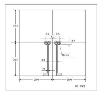
(2) Measurement condition Solder POSISTOR® on the substrate, then put a cover (150mm cubed) surround POSISTOR® to prevent flow of wind.
