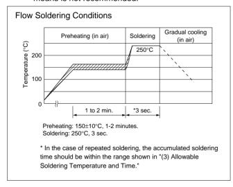
(5) There may be a risk of unexpected failures (tombstone, insufficient solder-wetting, etc.) in the mounting process caused by mounting conditions. Please make sure that this product is correctly mounted under the specified mounting conditions.
