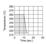
Allowable Reflow Soldering Temp. and Time
