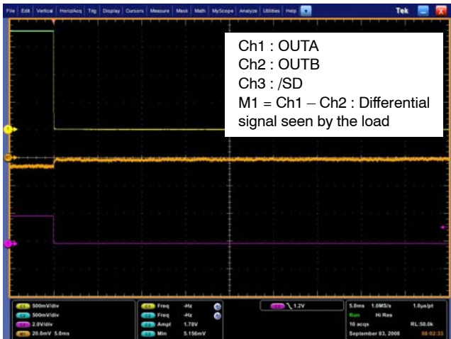
Figure 35. Zero pop noise turn off sequence with single-ended input to ground ( C_i = 47 \text{ nF} , R_i = 24 \text{ k}\Omega , R_f = 24 \text{ k}\Omega , C_{byp} = 1 \text{ }\mu\text{F} , R_l = 8 \text{ }\Omega , T_{on} = V_p )
